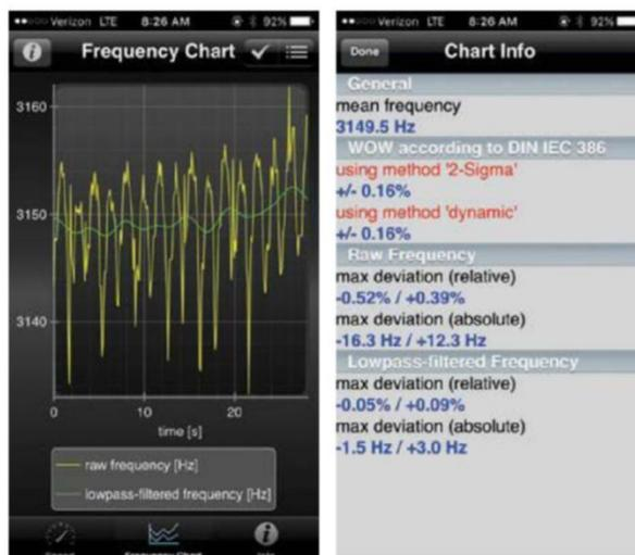
**Fig.1** (left) Soulines Kubrick DCX, speed stability (raw frequency yellow; low-pass filtered frequency green); **Fig.2** (right) Soulines Kubrick DCX, speed stability data.
